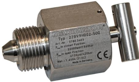
**Maximator** Bleed Valves are designed and engineered for use with Maximator Gauge Valves for high pressure venting before instrument calibration is performed. These valves can be purchased for both the sour gas and sweet service applications. Sour Gas applications where H<sub>2</sub>S is present, use the “SOG” suffix (22,500 psig).
