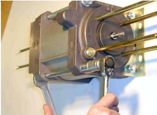
Remove the four hexagon nuts from the hexagon bolts.
