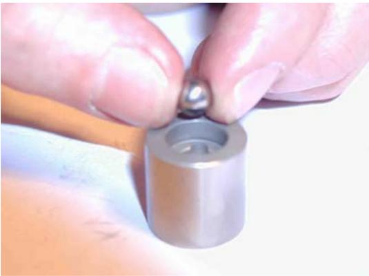
Place the ball onto the spring.
