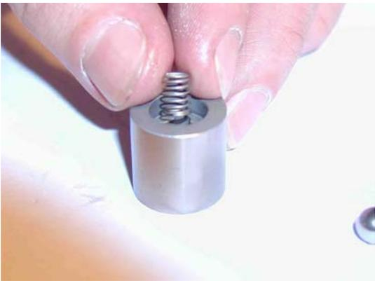
Insert the spring into the valve body.
