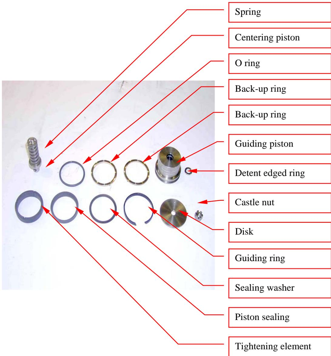
Remove the O ring and the back-up ring with a screwdriver from the guiding piston.
