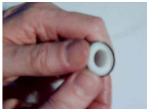
Grease the spool valve sleeve well, even when it is still installed. Insert the spool with rotating motions into the spool valve sleeve.
