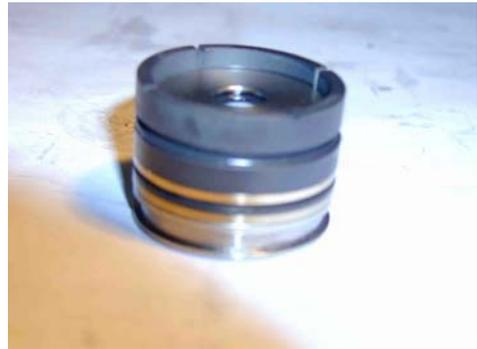
Grease the centring piston and attach its pertaining spring.
