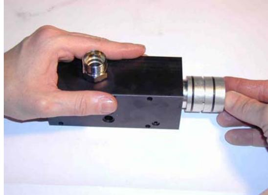
Re-insert the sealing cap into the spool valve housing and fasten it with the locking ring.
