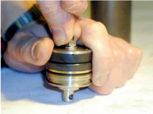
Compress the complete sealing package in anti-spring force direction. For the time being, tighten the castle nut only slightly (2-3 thread turns).
