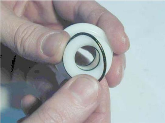
Then mount the two O rings into the grooves at the external diameter of the bushing.
