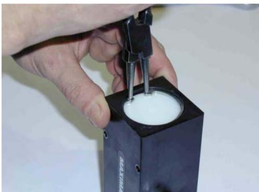
Dismantle the locking ring at the spool valve housing with suitable locking ring pliers. (The ring is located opposite the compressed air inlet).
