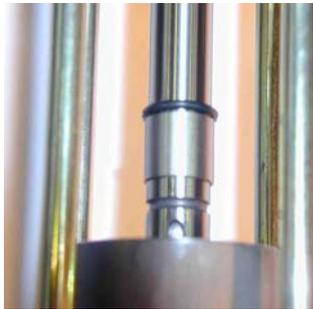
Move the O ring and the securing sleeve along the piston rod until the boring for the dowel pin is free.
