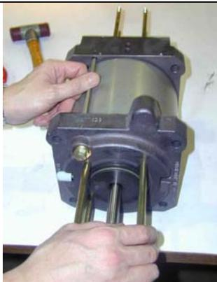
Slightly push the top and bottom cover together and insert the capillary control tube.
