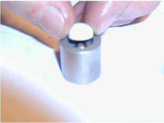
Place the valve seat onto the ball.
