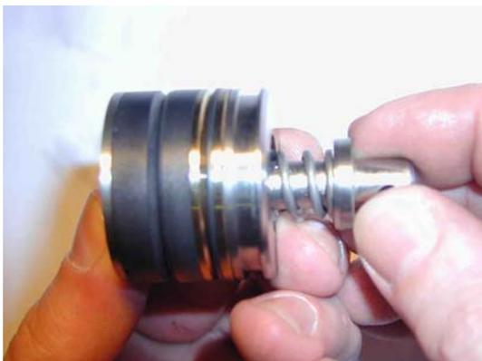
Place the disk on the tightening element and insert the centring piston into the guiding piston.
