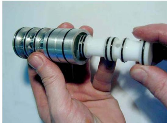
If applicable, grease the spool valve housing internally and install the spool valve sleeve with slight rotating motions into the spool valve housing.
