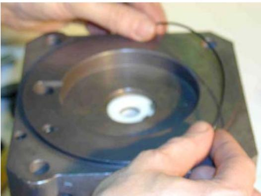
Mount the O ring that seals the air cylinder.
