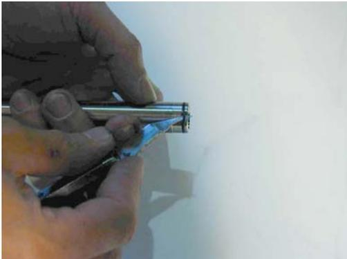
Remove the O rings from the pressure pipe.
