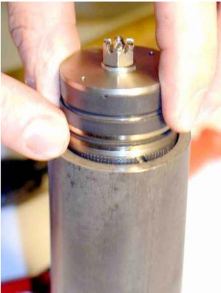
Insert the complete sub-assembly into the pressure cylinder. Check the correct seat of the guiding ring in the groove.
