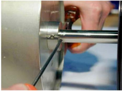
Safeguard the sub-assembly with the retaining pin.
