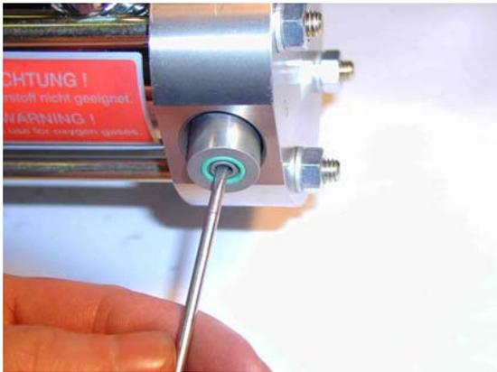
“Hook” the valves from the HP head with a screwdriver.
