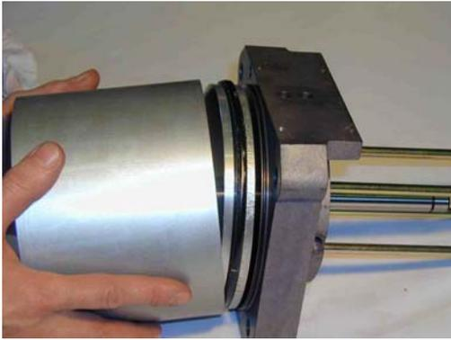
Withdraw the air cylinder from the top cover and the air piston.
